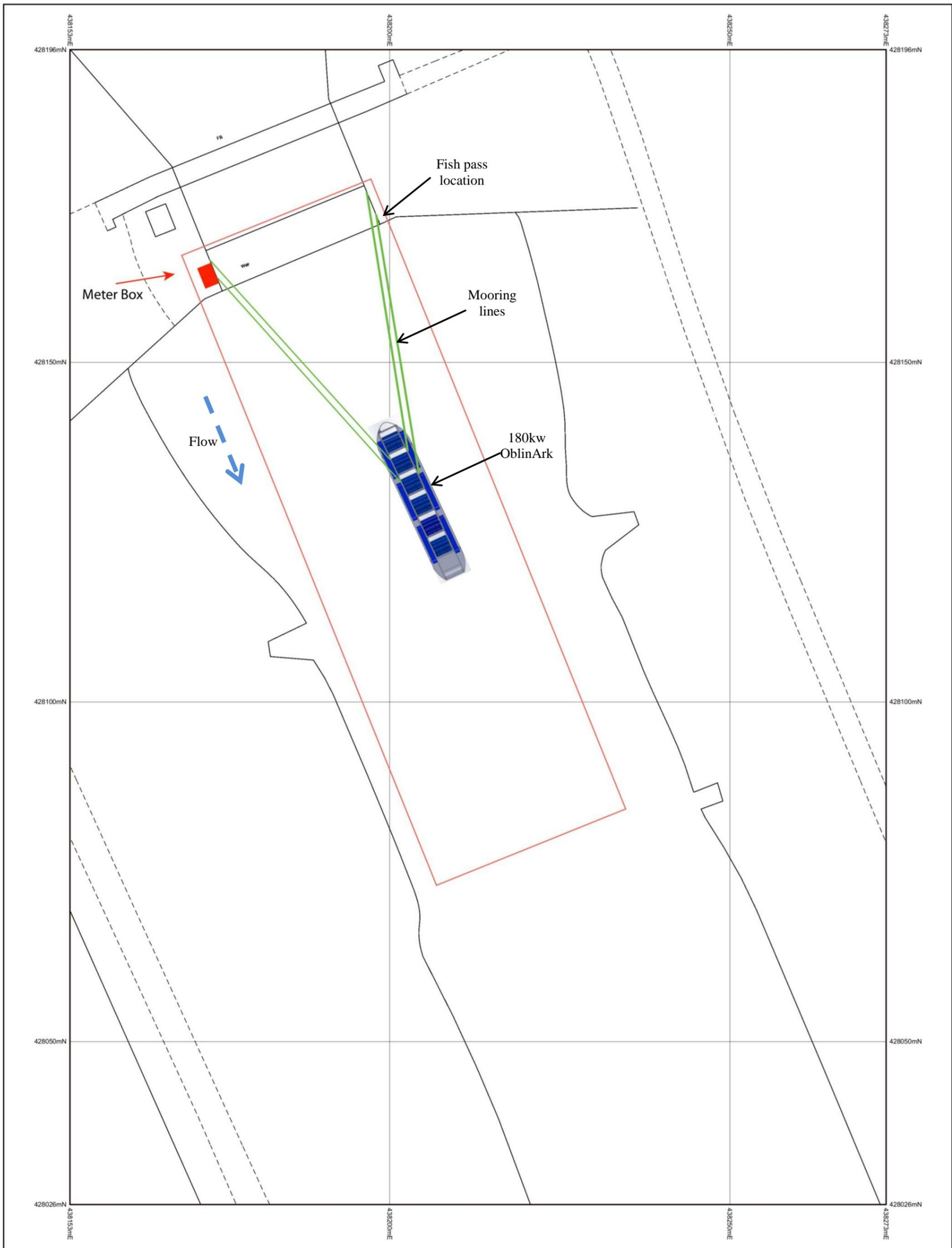
Figure 2. Plan view of the proposed installation of the OblinArk at Lemonroyd Weir (Courtesy of OblinArk Limited).
